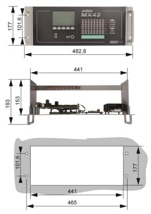
Figure 6: Size of the rack-mounted version.
