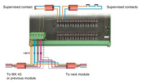
Figure 39: 16-logic input module connections.
