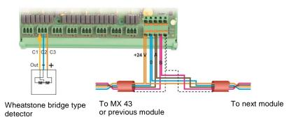
Figure 41: 8-analog input module connections for an explosive gas detection detector of the Wheatstone Bridge CEX 300 or OLC type.
