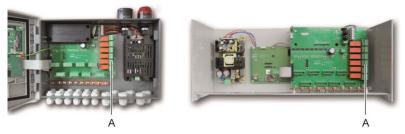
Figure 34: Internal alarm relay connectors (A).
