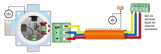
Figure 32: 4-20mA detector connected directly on the MX 43 channels.
