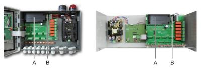
Figure 30: Positioning the battery pack.
