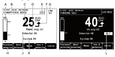
Figure 44: Example of the measurement display in normal mode and in inverse video.
