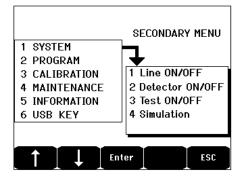
Figure 12: Example of a measurement display (screen) or parameter setting display (menu on the left).
