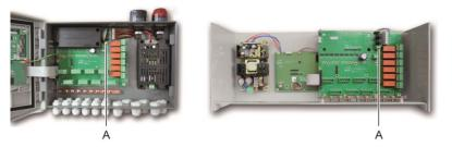
Figure 29: Connection of 24VDC external power supply (A).
