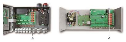
Figure 37: Location of the flash and siren connector (A).
