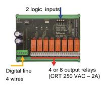
Figure 19: 8-relay module.
