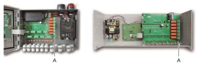
Figure 35: Remote acknowledgement connection (A).
