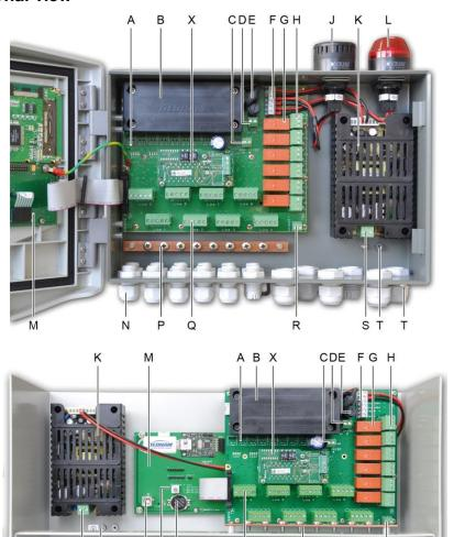
Figure 9: Internal view of the wall-mounted version (top) and rack- mounted version (bottom).
