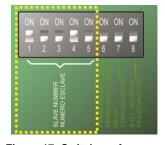
Figure 17: Switches of address configuration.
