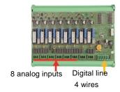
Figure 23: 8-analog inputs.
