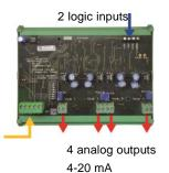
Figure 25: Principle 4-analog output module.
