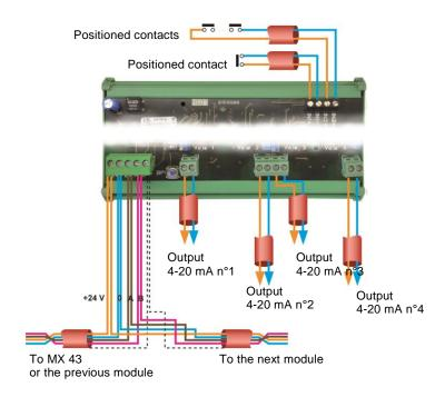
Figure 42: 4-analog output module connections.
